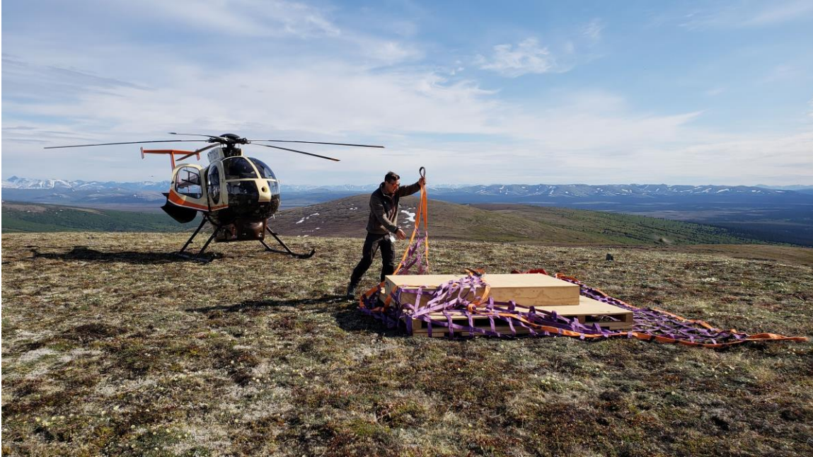
Figure 2. Helicopter sling load operation performed by pilot.
