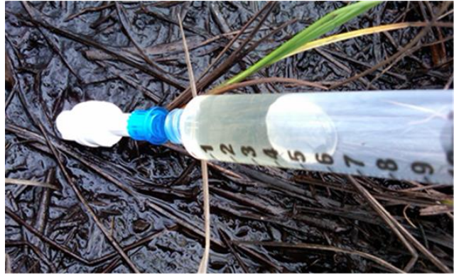
Figure 4. A syringe is used to extract water samples from permafrost soils.
